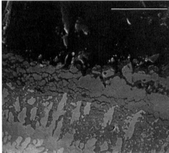
FIGURE 13 SEM image in secondary electron mode. Al – 4 (at.%) Ru alloy showing the cascade of peritectic reactions, forming \text{Al}_3\text{Ru}_2 , \text{Al}_{13}\text{Ru}_4 and \text{Al}_6\text{Ru} . From bottom left-hand corner: \text{AlRu} dendrites (lightest), \text{Al}_3\text{Ru}_2 dendrites (light grey), \text{Al}_{13}\text{Ru}_4 layer (medium grey), \text{Al}_6\text{Ru} (dark grey) with (Al) matrix (black) [37]. Bar represents 50 \mu\text{m} .
